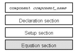
The equation section of a Simscape file follows the declaration and setup sections. It is executed throughout the simulation. The purpose of the equation section is to establish the mathematical relationships among a component's variables, parameters, inputs, outputs, time and the time derivatives of each of these entities.
